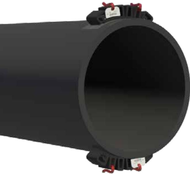
The restraint is a flexible bar, which is fused to the pipe by electrofusion to create a welded shoulder that can restrain the axial movement of pipes in various applications:
